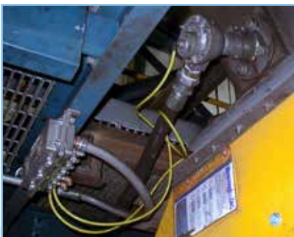
PACS is the only radial, pneumatic cleaning system specifically designed for bulk material handling and designed to not damage ceramic-lined chutes.
