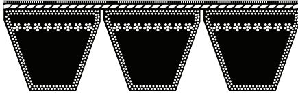
Envelope 5V, 8V Cross Section
